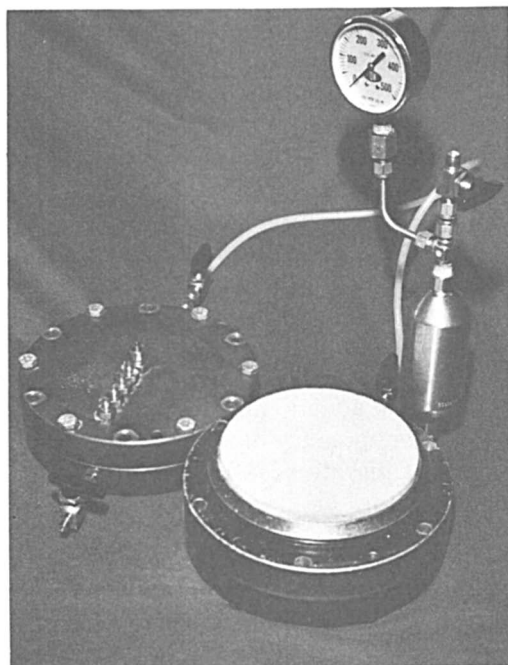
Figure 11. Disk in holder for radial flooding.
